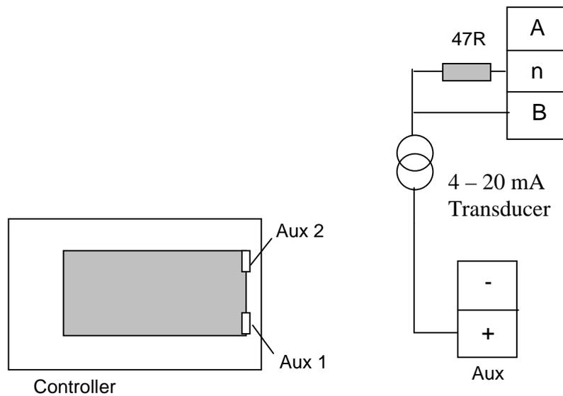
Note that Auxiliary 1 is powered from the backup battery (if fitted) in the case of a power failure, whereas Auxiliary 2 is not.
