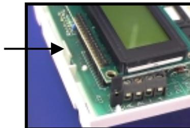
3. Mount the back cover of the keypad, using the four slotted holes.
