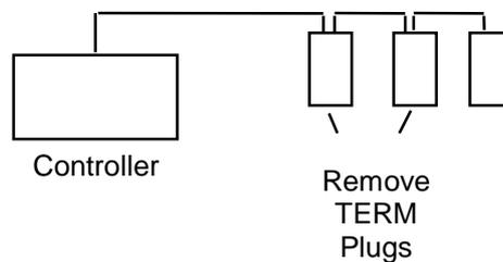
You now need to set the addresses of the keypads. Provide power to the keypads (by powering up the controller or an external supply if applicable).
