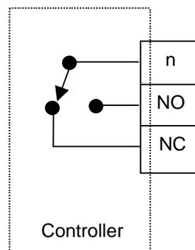
The rating is 1 amp maximum switching with the maximum voltage depending on whether the application is required to meet UL approval:
