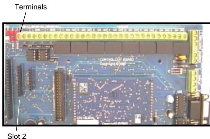
Connect the controller into the C-Bus via the C-Bus terminals on the top left of the controller board (indicated above).
