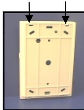
2. Turn the keypad on its back and remove the circuit board by pushing back the clip holding the top of the board.
