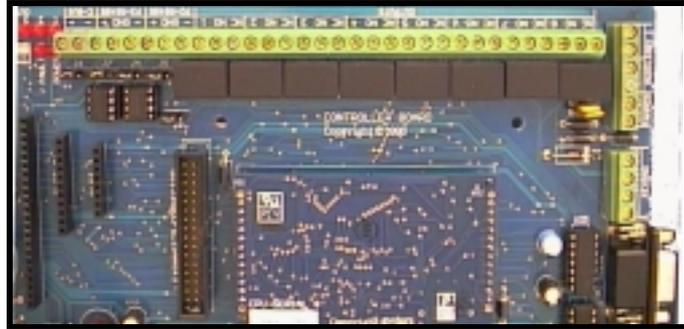
Each output has a numbered terminal and NC (Normally Closed) and NO (Normally Open) terminals. These are connected internally to a relay as shown below.
