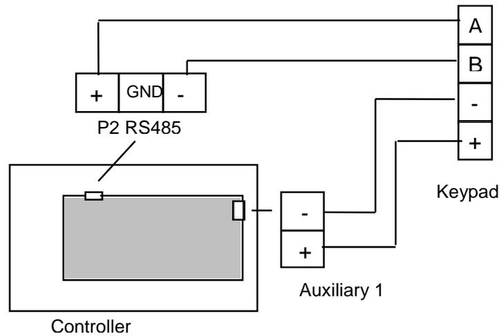
Do not connect the shield at the keypad.
