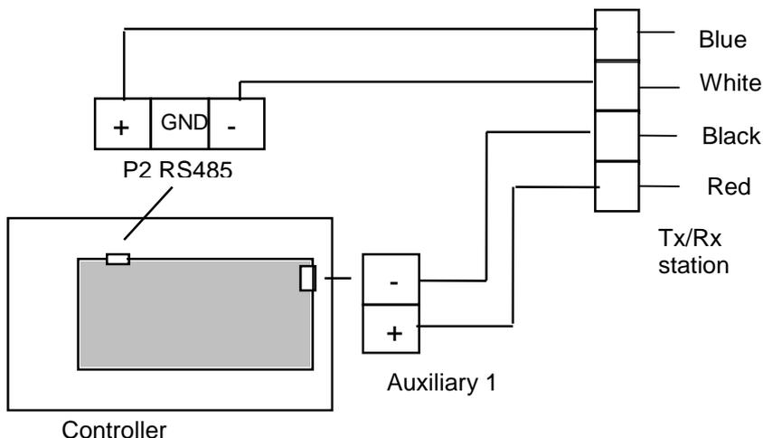
You can connect other stations by extending the wiring from each station to the other.
