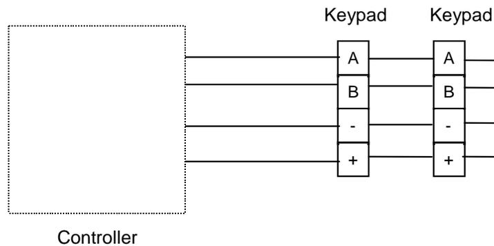
On all except the last keypad, remove the shorting plug from the TERM socket, which is located just above the terminal block.
