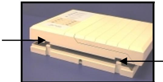
2. Mount the back with screws through four of the slotted holes.
